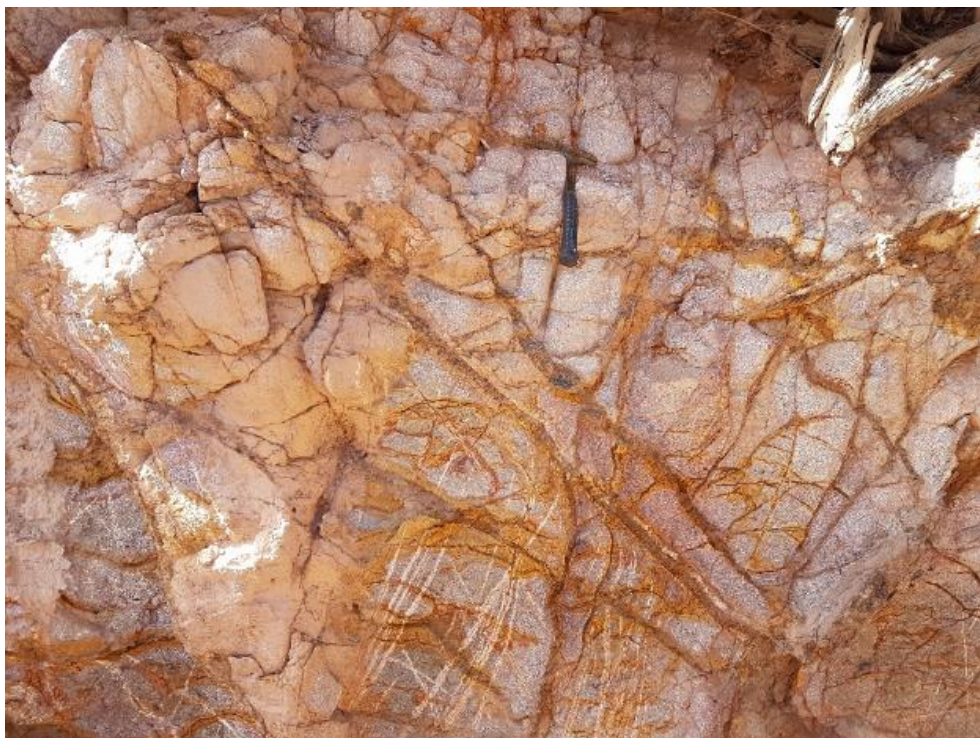
Figure 2 Stockwork quartz veining and selvage alteration within dolerite at the Agnes Prospect
