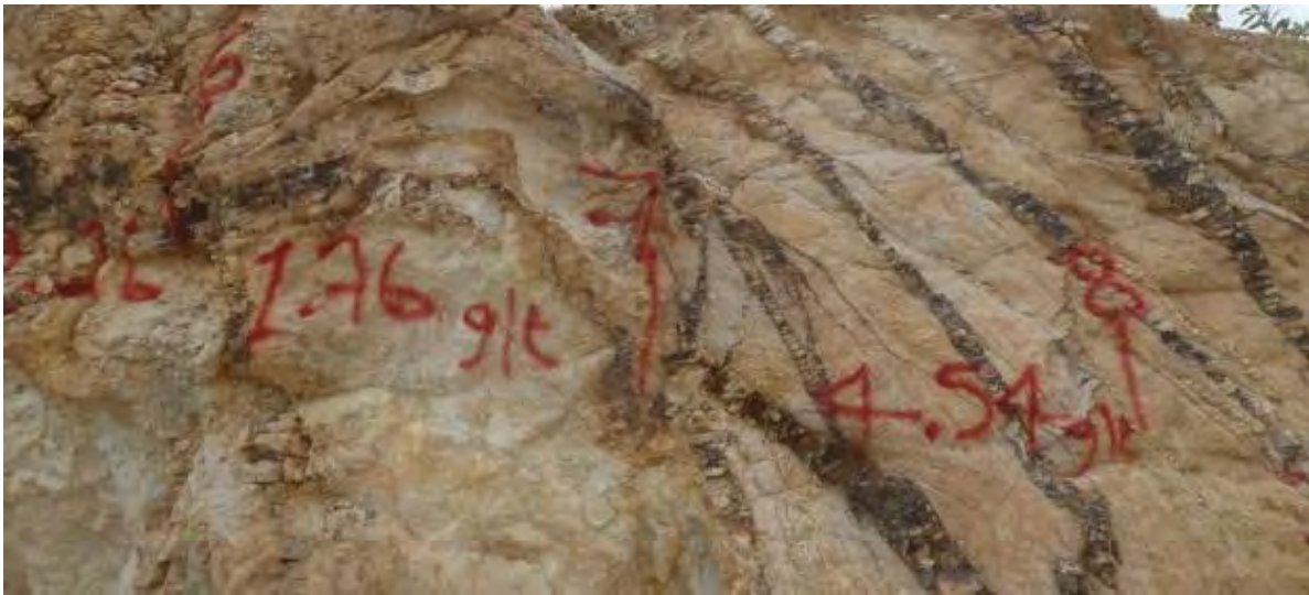
Portion of channel sampling traverse, showing sheeted to stockwork quartz veining within the porphyry host and 1m channel sample grades marked on the face.
