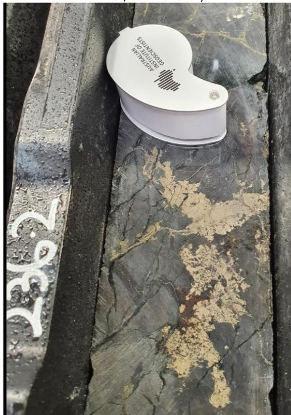
The photo of the core from Government drill-hole NDIBK04, shows core at depth 236.2m . The core has been cut in half and one half has been cut again. A quarter-core sample every metre has been submitted for multi-element analysis.
